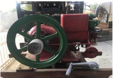
1920, International M, 1 1/2hp, very complete, over strike ignitor, mag puts out some voltage, fires on battery and coil, original hand crank, gas or kerosene carb.
