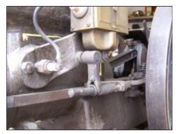
The pushrod was pretty much rusted so I had my friend and WAPA member Dale Linn make me a new one using the old one as a pattern. So it would not rust, I took it to work and put it in with the other parts going out for nickel plating. The mag trip rod and springs were badly rusted so I replaced them with a threaded rod and springs from McMaster Carr.
