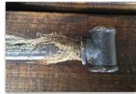
After assembly, you'll need to trim the excess flax using a sharp blade.
