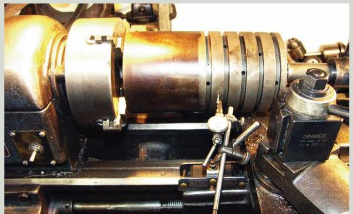
With the piston running perfectly true, I need to run a center in the tailstock to hold the end of the piston. There is already a center hole from when the piston was manufactured, which will save the trouble of having to lay out the exact center and drill my own hole. Because I will be using a dead center, the hole needs to be lubricated with white lead or another suitable compound.
