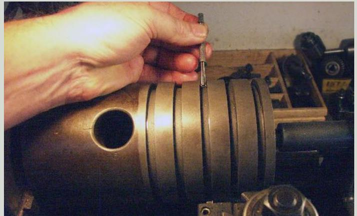
Upon finishing all five grooves, I leave the piston in the lathe and install the rings. To my dismay, the grooves that provide less than 0.001 inch clearance are too tight. I now go back and open up the tight grooves a little, re-install the rings, and everything now looks good.
